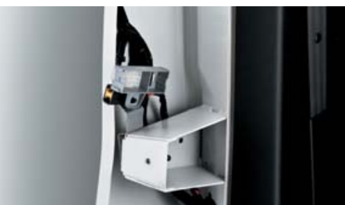
Transformer socket - electrical interface for connecting body equipment services (opt. 081)
